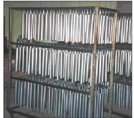
Parts can be densely racked for treatment in the dip tank.
